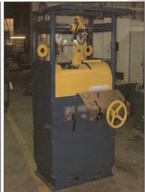
Rig powered hydraulic unit with manual levelwind (25,000 ft. of 0.092" wire).
