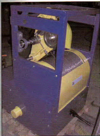
Low profile AC vector driven system with automatic levelwind (15,000 ft. of 0.108" wire).
